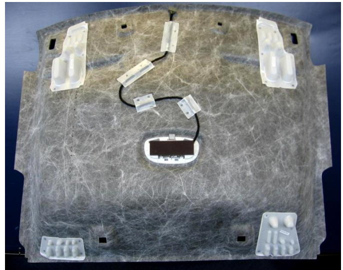
Figure 3. HIC and wire retention clips secured to headliner by InfraWeld process
