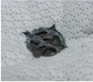
Figure 8. Close-up of NVH pad, InfraWeld spot-weld
