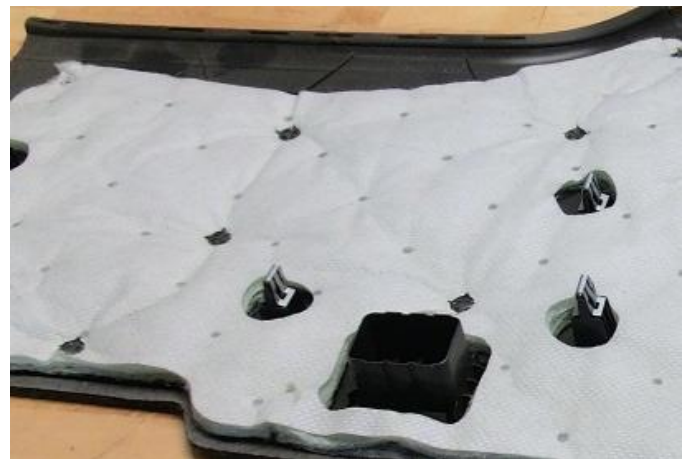
Figure 7. NVH pad bonded to trim panel with the InfraWeld process
