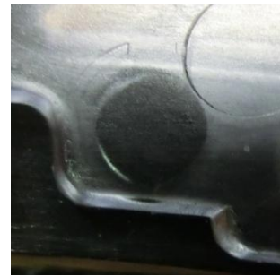
Figure 6. Close-up of polycarbonate spot-weld with the InfraWeld process
