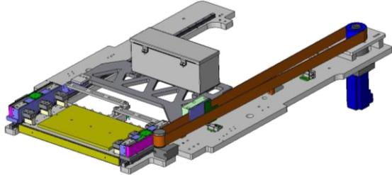
Figure 3. *Rapid Conductor Heat Platen Spatial Compensation Design*
