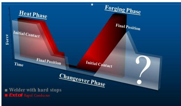
Figure 2. Force vs. Weld Time Graph.
