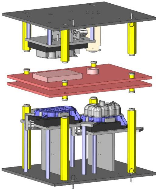
Figure 1. Traditional hot-plate weld tooling depicting a two-place set assembling two halves of a Tank on the left side and a small Fill Neck detail on the right
